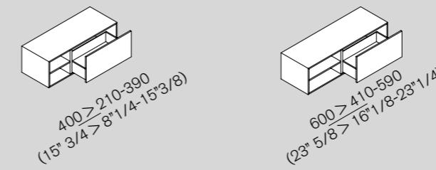
Besides the standard measures, the compositions with 1 open storage unit are possible with custom made measures too. The open storage unit of 40 cm (15" 3/4) may have custom dimensions that vary from 20 (7" 7/8) to 39 cm (15" 3/8), the storage unit of 60 cm (23" 5/8) from 41 (16" 1/8) to 59 cm (23" 1/4).
