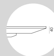
The edge of the Ell countertop aligns itself to the different necessities of use with several formal proposals. Tapered on the three visible sides in the self-supporting version, with shaped edge for the version that rests on cabinets.
